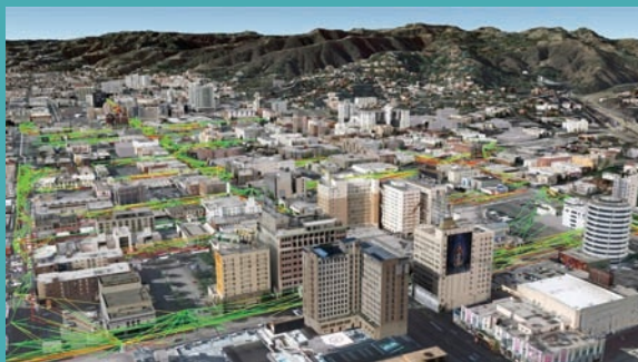
Figure A Streetline Networks' smart-parking management solution uses Linear Technology/Dust Networks' wireless technology in a wireless mesh network overlaid on urban streets. Wireless sensors buried in the pavement gather information on parking-space availability that is sent wirelessly to smartphone users.
